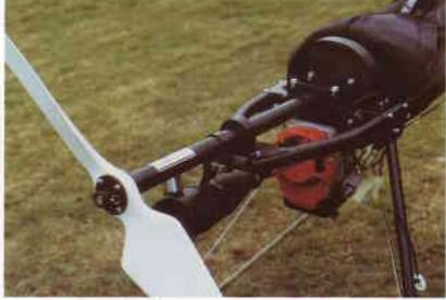
At the top is Tomas Oiala from AcroSport ready to start his Mosquito. Note the position of the tank and shortened keel of the wing. The landing gear makes it very easy to walk with the unit on the ground.
